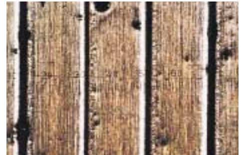
Typical wedgewire element—approximate void volume = 4%.
