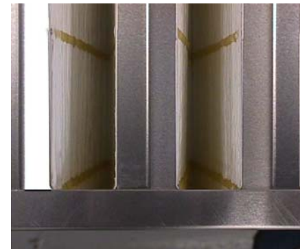
Used CAF, downstream after 14 months service
