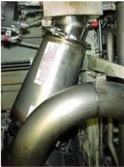
Photo: Pall F100 bleed air filter
